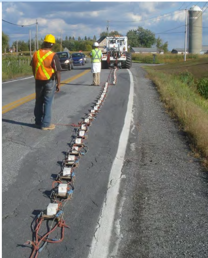
Minivib-landstreamer data acquisition system in operation (Photo from A. Pugin).
