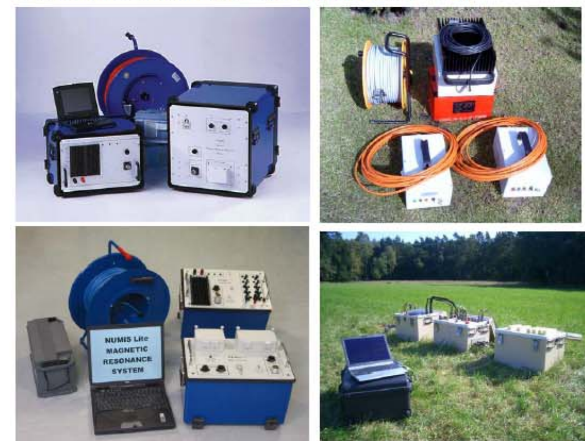
Figure 5: MRS implementations: top left: original NUMIS, top right: Radic SNMR MIDI, bottom left: NUMIS LITE , bottom right: GMR, Clara Vista.
