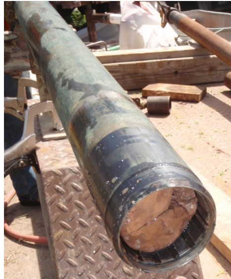
Triple-tube core barrel
